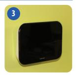
Once clipped into place, ensure the unit is securely seated on the bracket.
