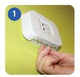
Using a paper clip, insert into the hole marked SYNC at the bottom of the iT500RX Receiver. Then work through the screen sequence shown on the next page.
