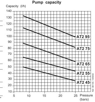
Viscosity = 5 cSt - Rated speed = 2850 rpm Data shown take into account a wear margin. Do not oversize the pump when selecting the gear capacity to ensure the optimum operation of the (NO) solenoid valve (switching low/high mode).
