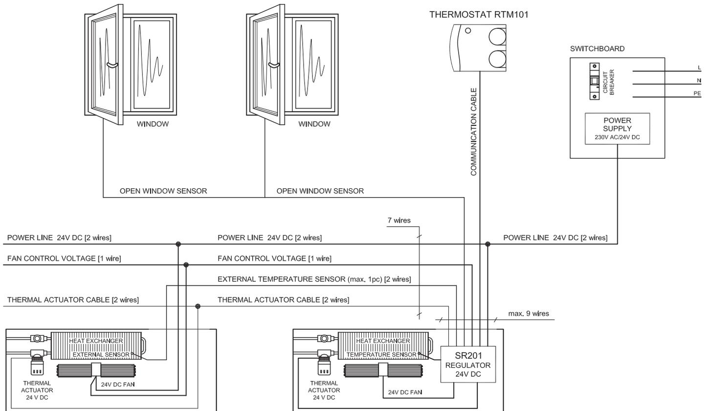
For current installation, you only need 1 thermostat, 1 regulator and 1 power supply unit per a room. In case of extended projects, where the power input of installed convectors goes beyond 100W, an additional regulator and a stronger power supply unit is to be installed. Please contact the manufacturer.
