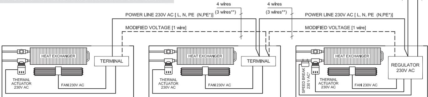
\* installation of the speed break only to the first convector
