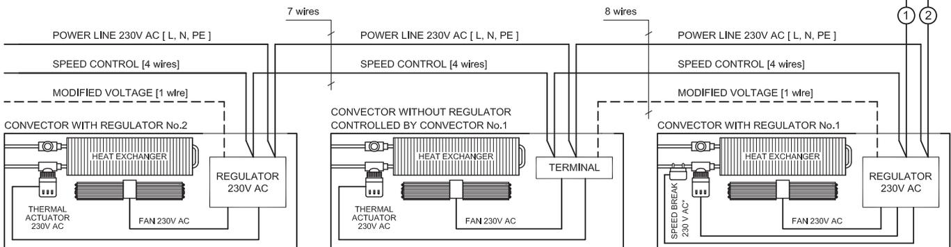
\* installation of the speed break only to the first convector
