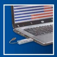
You also have the possibility to use our *PROGmatic* stick for transferring your individual heating- and saving-times quickly and easily to the *comet*. Simply connect PROGmatic to your PC. Using the software stored on the stick, you can define your heating and saving times. Then you insert your PROGmatic device into your energy-saving controller to copy the individual room profile created on your PC.
